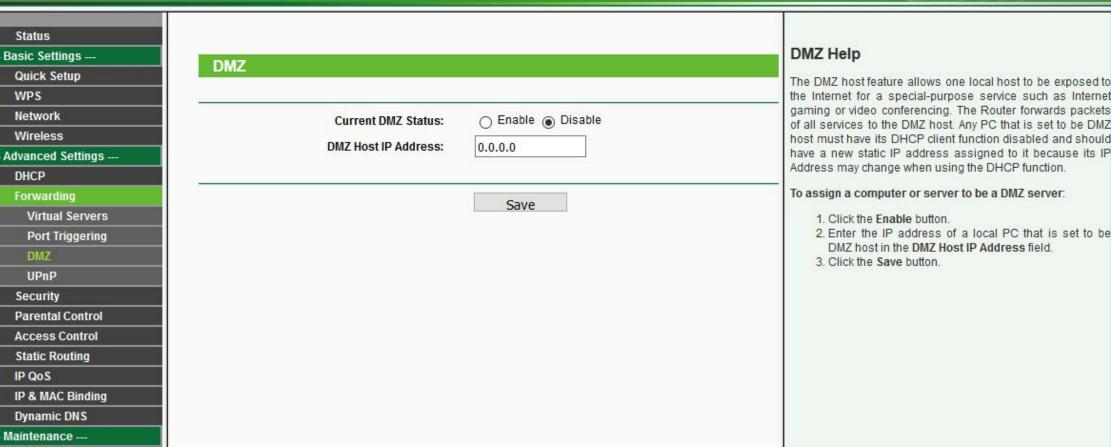
The DMZ host feature allows one local host to be exposed to the Internet for a special-purpose service such as Internet gaming or video conferencing. The Router forwards packets of all services to the DMZ host. Any PC that is set to be DMZ
